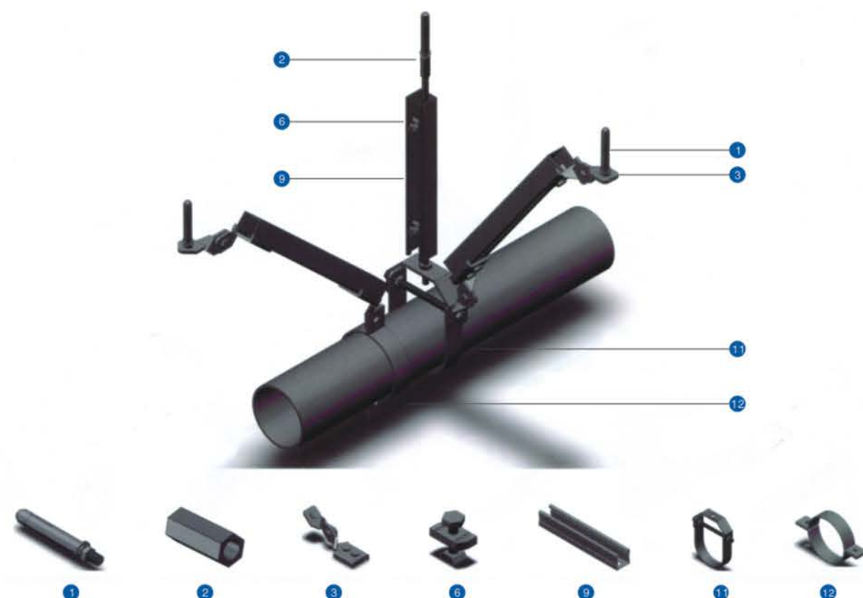
Single pipe- longitudinal seismic support. ( Pipe lifting height 1 meter )
